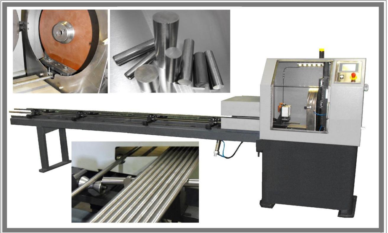
Fully AUTOMATIC ABRASIVE CUTTING MACHINES Type ASM with Bar Magazine, Automatic Feeder and Touch Panel for the accurate abrasive cutting of harden steel and other exotic materials with an accuracy of +/- 0,05mm (.002"). All machines are easy and quick to set up and can adapt cutting-wheels of up to 300 mm (12 "), have automatic surface speed adjustment control and will also adjust the cutting position to compensate for wheel wear in order to reduce valuable production time.
